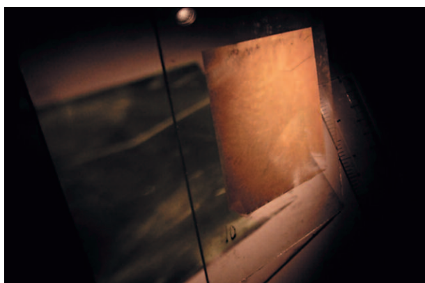
Fig. 1. A 3" x 3" gold leaf mounted on glass by Faraday. The light source is on the right. Reflected light is gold in color while that transmitted through the leaf is green. Courtesy of the Royal Institution.
