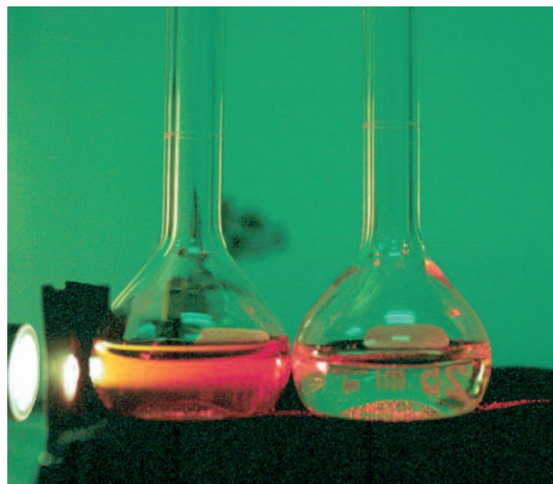
Fig. 4. One of our "citrate" gold colloids (left), and a solution of gold chloride (right). The narrow beam of light shows the "Faraday-Tyndall Effect" on the colloid but not the solution.
